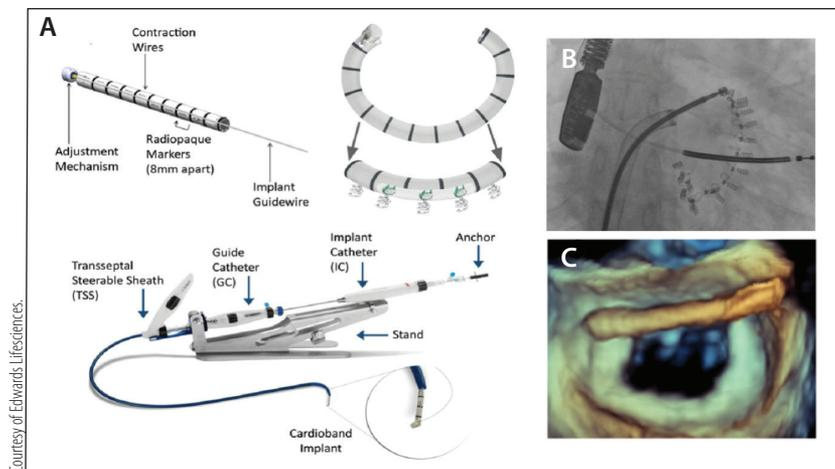
Figure 5. Cardioband direct annuloplasty and delivery system (A). Fluoroscopic (B) and echocardiographic (C) appearance of Cardioband implantation.
